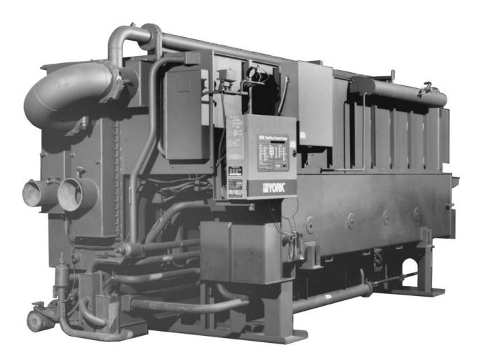
The YORK YPC Two-Stage Absorption Steam Chiller represents the world's most efficient commercially available absorption technology. The unique Two-Stage design requires a remarkably low steam input rate of 9.8 lbs. per ton-hour (1.26 kg per kW-hour), which equates to a COP of approximately 1.19. With today's energy and environmental considerations, the YORK YPC Two-Stage Steam Absorption Chiller is the ideal choice for a wide range of applications.
