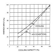
FIG. 1 - ENERGY INPUT VS. OUTPUT
