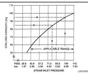
FIG. 3 – CAPACITY VS. INLET STEAM PRESSURE AVAILABLE
