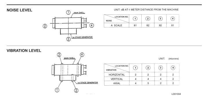
**FIG. 2** – TYPICAL NOISE AND VIBRATION LEVELS JOHNSON CONTROLS
