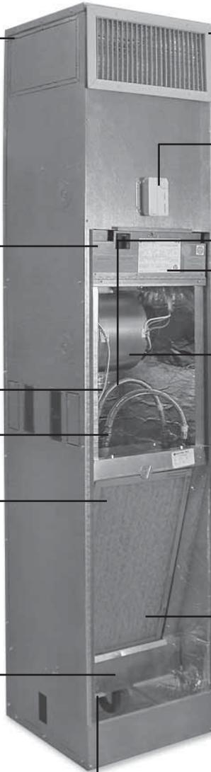
Tandem Master and Tandem Slave Models FSA/FSB ship complete with risers enclosed in a wall plenum with one layer of 5/8" gypsum for sound attenuation. As an option, Tandem Master and Tandem Slave units may be ordered with two layers of 5/8" gypsum and fire blocking material for a one hour fire rating per UL 1479.
